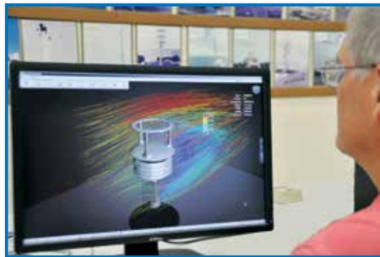
The design of the Response ONE™ was analyzed using computer aided engineering (CAE) tools including computational fluid dynamics (CFD) modeling.
