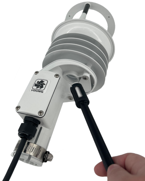
2. Unscrew filter and remove
