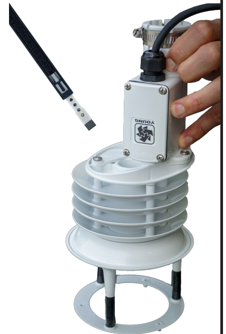
3. Pull out sensor stick with sensor stick tool
