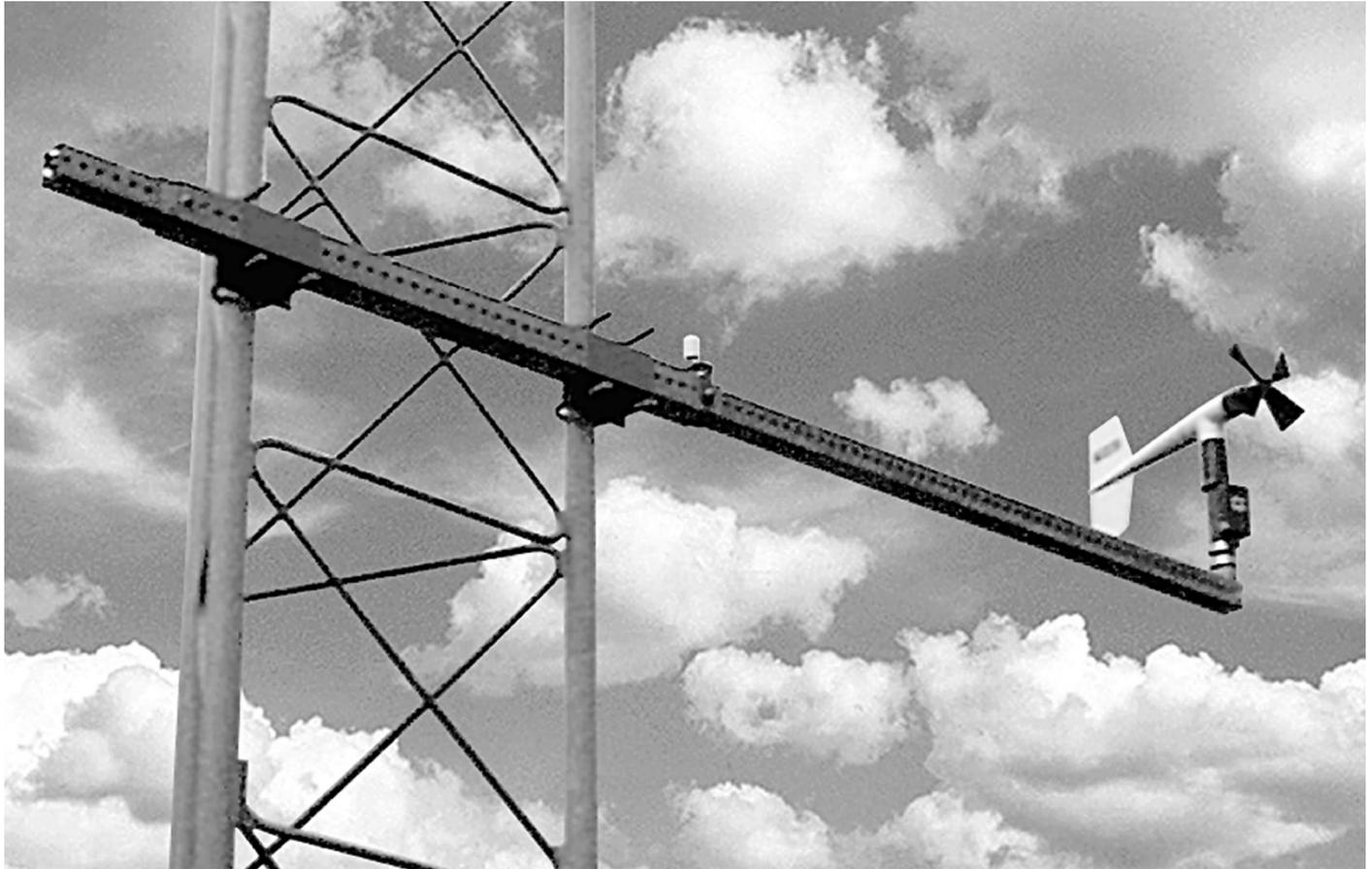
**Retractable Mounting Arm** allows rigid mounting of instruments away from tower to minimize effect of the tower structure on measurements. Tele-scopic design retracts for easy installation and service of sensor. Constructed of galvanized steel square tubing, the mounting arm is supplied with universal mounting brackets that bolt to tower legs. 1" IPS mounting post fits YOUNG sensors.
