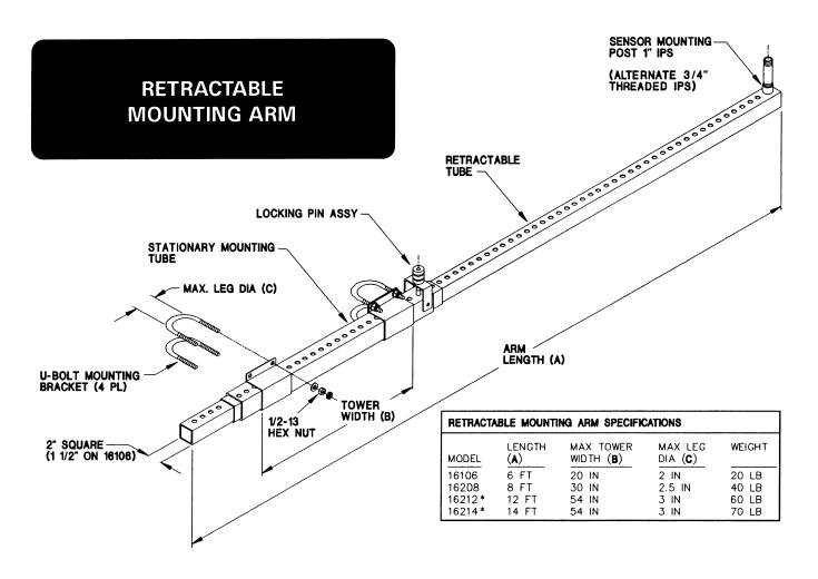
**Retractable Mounting Arm.** Galvanized steel telescoping arm provided with universal mounting brackets for bolting to side of tower. Allows rigid mounting of instrument away from tower to minimize effect of tower structure on wind measurements. Retracts for installation and service of sensor. Includes 1" I.P.S. mounting post for sensor.
