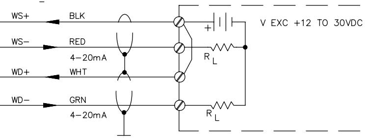
$$\text{MAX LOAD RESISTOR } (R_L) \text{ VALUE} = \frac{V_{EXC} - 12}{0.02} = R_L$$
