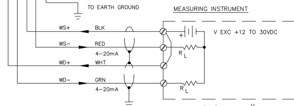
MAX LOAD RESISTOR ( $R_L$ ) VALUE =  $\frac{V_{EXC} - 12}{0.02} = R_L$
